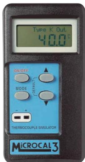
The MicroCal 3 has 23 fixed temperature points for type K thermocouple -100, -50, -20, -10, 0, 10, 20, 30, 40, 50, 60, 80, 100, 150, 195, 250, 300, 400, 500, 600, 800, 1000 and 1200 °C.
