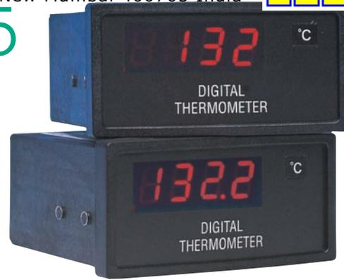
The Therma D81 and D85 panel thermometers offer high accuracy with excellent long term stability. The large, 3½-digit LED display offers a wide temperature measurement range with clear indication of readings and a choice of 0.1°C or 1°C resolution. The thermometers are housed in a 48 x 96mm DIN size, glass-filled plastic case with a minimal 88mm behind the panel space requirement.
