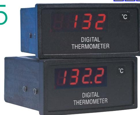
The Therma D41 and D45 panel thermometers offer high accuracy with excellent long term stability. The large, 3½-digit LED display offers a wide temperature measurement range with clear indication of readings and a choice of 0.1°C or 1°C resolution. The thermometers are housed in a 48 x 96mm DIN size, glass-filled plastic case with a minimal 88mm behind the panel space requirement.
