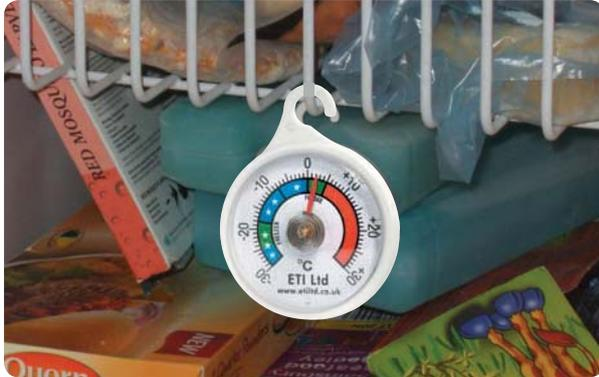
This easy to read fridge/freezer thermometer has a Ø52 mm dial. The thermometer indicates temperature over the range of -30 to 30 °C in 1 °C divisions.
