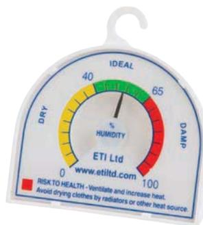
This room hygrometer incorporates a 70 mm diameter dial with colour-coded zones indicating the moisture/water vapour in the atmosphere. The unit indicates the level of humidity in 5 % divisions over the range of 0 to 100 %rh. The ABS housing measures 70 x 60 mm and can be free-standing or hung from a shelf.
