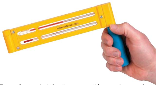
This professional whirling hygrometer (sling psychrometer) offers a means to accurately measure the relative humidity utilising wet and dry bulb spirit-filled thermometers. The unit incorporates a water reservoir linked to the wet bulb by the means of a cotton sleeve.
