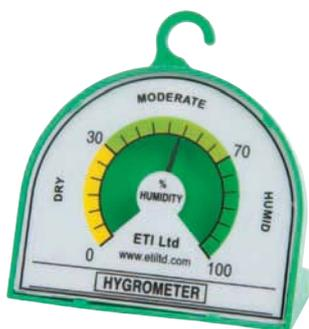
This easy to read, general purpose, hygrometer incorporates a 70 mm diameter dial with colour-coded zones. The hygrometer indicates the level of humidity in 5 % divisions over the range of 0 to 100 %rh. The green ABS housing measures 70 x 60 mm and can be free-standing or hung by the hook from a shelf.
