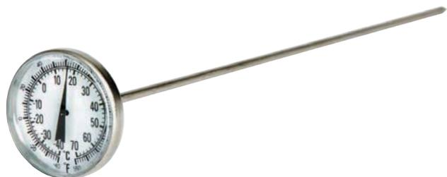
This simple to use Ø45 mm dial probe thermometer is reliable and accurate. The hot water dial thermometer features a Ø4 x 300 mm pointed stainless steel stem. The thermometer indicates temperature over the range of -40 to 70 °C in 2 °C divisions.
