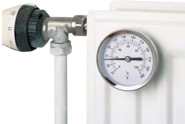
This Ø60 mm stainless steel surface dial thermometer incorporates a magnetic sensing pad for mounting on ferrous metals and indicates temperature ranges 0 to 120 °C.
