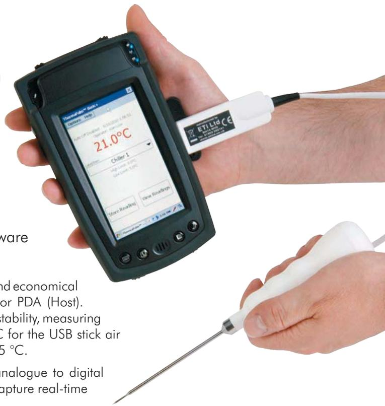
The Precision USB Thermometer Probe provides a reliable and economical method of measuring temperature utilising a computer or PDA (Host). Each probe is calibrated to provide excellent accuracy and stability, measuring temperature over the range of -40 to 125 °C (0 to 70 °C for the USB stick air probe) with an 0.1 °C resolution and an accuracy of ±0.5 °C.
